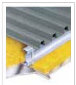
The roof cladding should be carried out in conjunction with the insulation work to avoid accidental damage. Fixing should be through the crown profile of the roofing sheet and down through the spacer to the purlin below.
