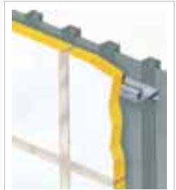
As an alternative to the above, timber packing strips may be cut to suit the sheeting rails and screwed in place, fix the KIMMCO Building Roll at the head of the wall by screws into the timber packer with a steel strip placed on top of the insulation directly over the packer. Repeat as required at other sheeting rail locations, ensuring that the KIMMCO Building Roll are closely butted to each other with the edge flanges overlapping.
