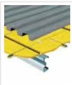
b) Alternatively, the insulation can be applied from rolls initially secured at the ridge and allowed to unroll progressively towards the eave in conjunction with the application of lining boards. It is important that the adjacent layers of insulation are sufficiently overlapped to prevent heat loss or gain.
