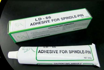
Manufactured using synthetic rubber, BRG Adhesive LD-66 is designed for use with BRG Spindle & Hanger to provide fast bonding for applications such as fixing of Metal Lath/Strip Mesh onto wall prior to plastering in particular crack-prone areas between concrete and brick/block work; as well as for fastening of fiber-glass wool in hot and cold insulation works. Other applications include the fastening of BRG mesh products.
