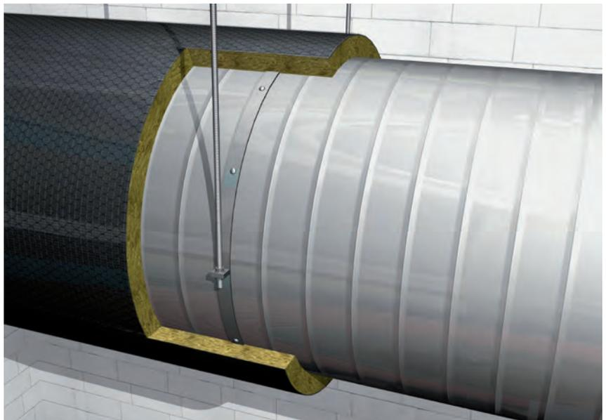
*Installation principle for horizontal circular ducts*
