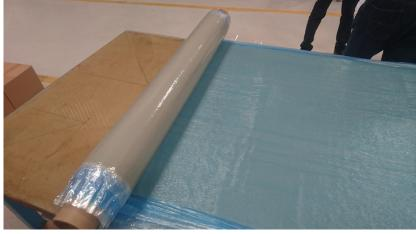
SolarLine GRP is a soft, mouldable material held between two barrier films. SolarLine GRP can be easily cut with scissors or a modelling knife.
